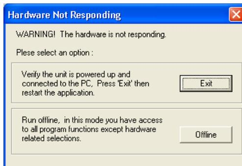
You have the option to exit and correct the hardware connection or continue and execute the software in offline mode. When choosing 'Offline' the software will execute normally except that any menu selections or toolbar buttons which control hardware will be disabled.
