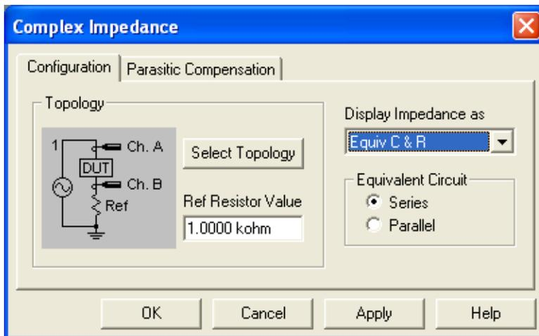
When the 'Select Topology' button is clicked the topology selection dialog is displayed which displays six configurations for Device Under Test (DUT) connections. Choose the topology which matches your setup. The 'Select Topology' and 'Parasitic Compensation' dialogs are shown below.
